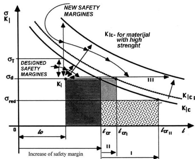
Fig.1. Illustration of appliance of general criteria for increase of safety of fatigue fracture [1] and [3]
