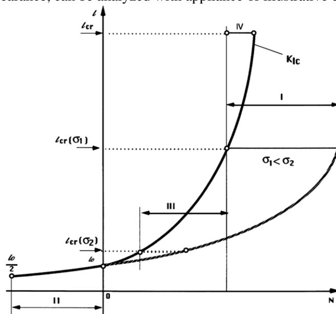
Fig.2. Illustration of primary factors for fatigue fracture control [1] and [3]
