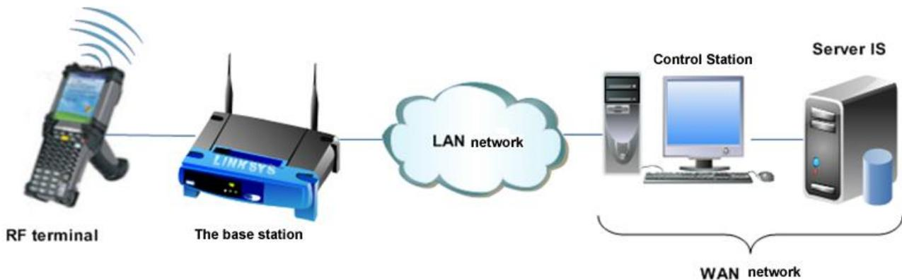
Figure 3 – The working principle of RF terminals
