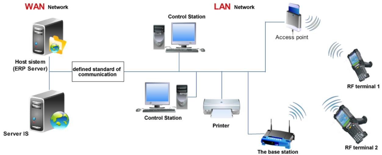
Figure 2- IS network architecture for storage
