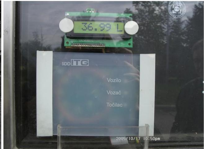
Fig. 4 Detailed view of ID card reader's antenna
