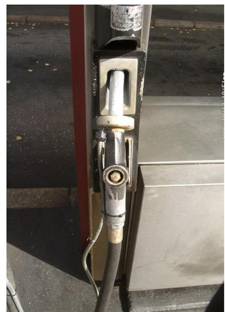
Fig. 2 Pump nozzle with antenna for vehicle identification
